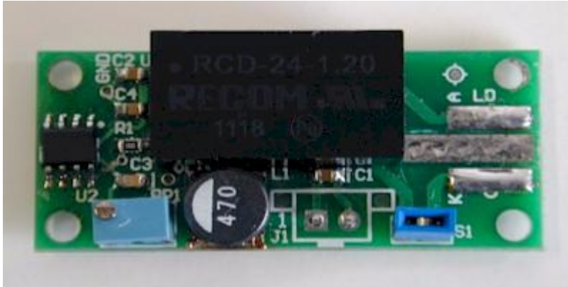
Figure 1. OELDD-400, 15V laser diode driver
